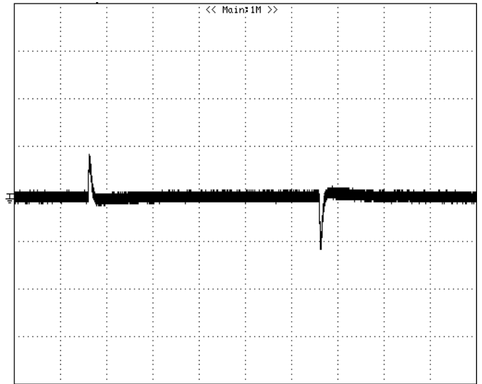
Figure 22: Typical transient response to step load change at 1A/\mu S from 100%~ 50%~100% of I_o , max at 12Vin, 1.8Vout ( C_{out} = 1\mu F + 47\mu F + 10\mu F ceramic) CH1 : VOUT, 0.1V/div, 200uS/div
