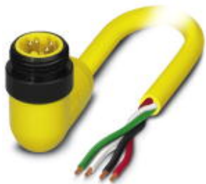
Power cable, 4-position, PVC, yellow, Plug angled 7/8"-16UNF, A - standard, on free cable end, A - standard, cable length: 2 m
