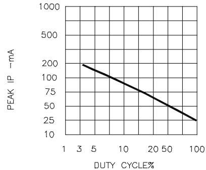
DUTY CYCLE% Fig.6 MAX PEAK CURRENT VS. DUTY CYCLE (REFRESH RATE f=1KHz)
