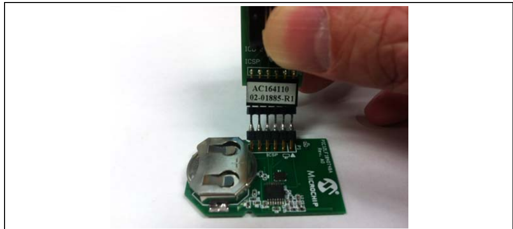
FIGURE 6-1: PROGRAMMING THE KEY FOB
