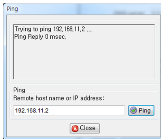
Figure 6. Simple Ping Test Program
