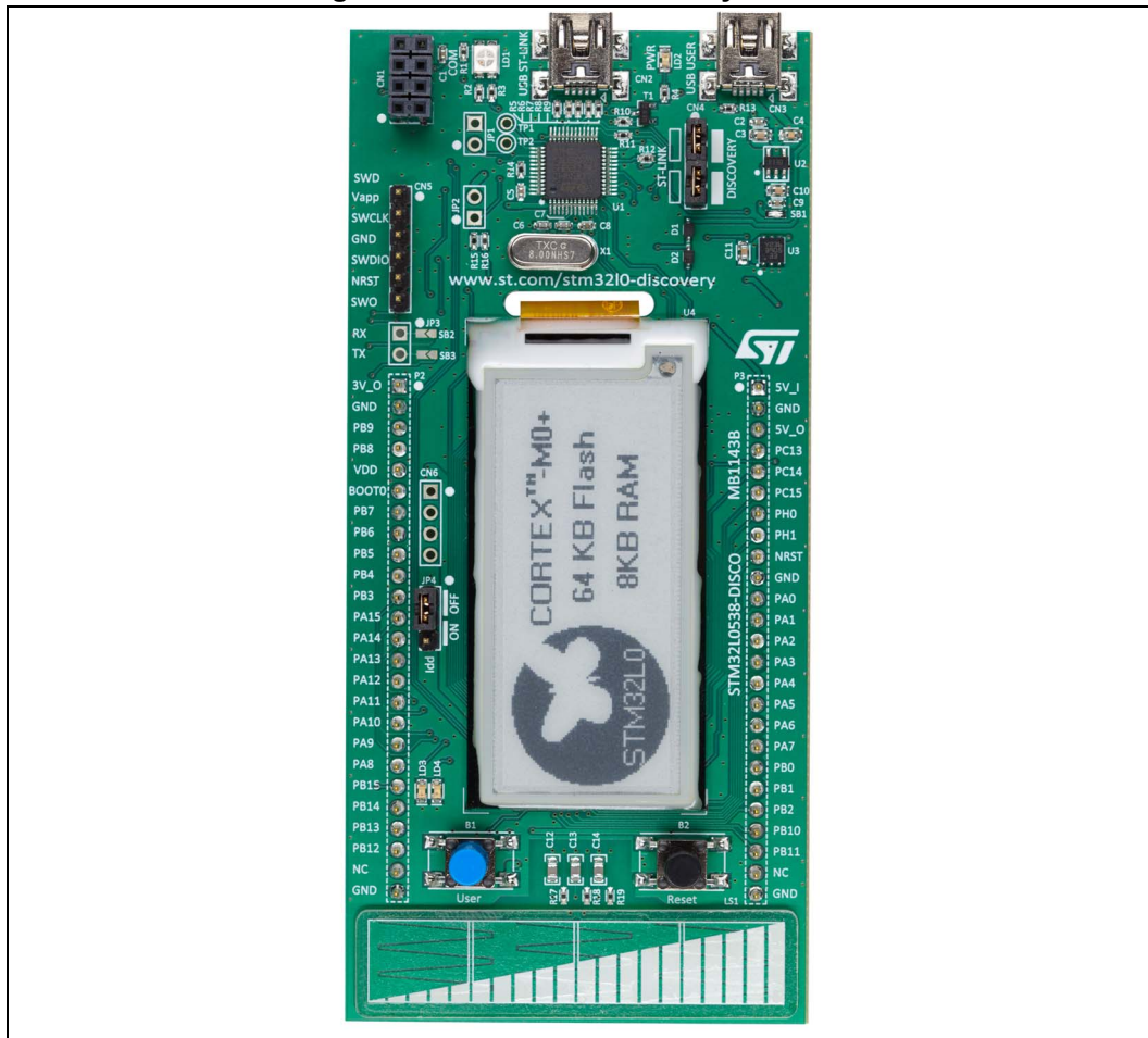
Figure 1. STM32L053 discovery board
