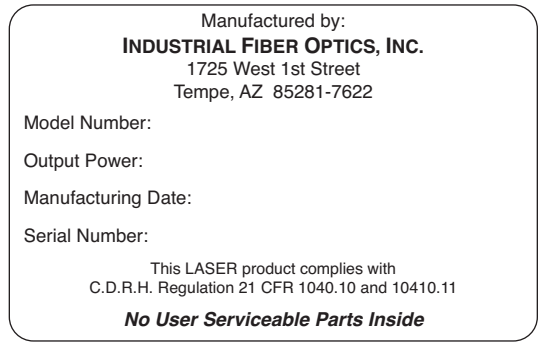
Figure 3. Laser certification and identification label.
