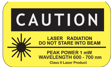
Figure 4. Warning logotype label for Class II lasers.
